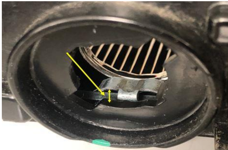
Figure 1. Tail lamp contact loose/pulled away from housing.
