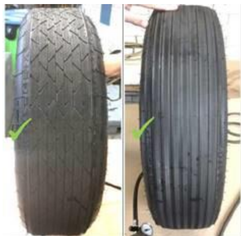
Figure 1. Correct tire position – tread aligned symmetrically with the rim/hub.
