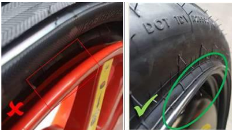
Figure 2. Tire assembly; Incorrect and correct positions shown.
