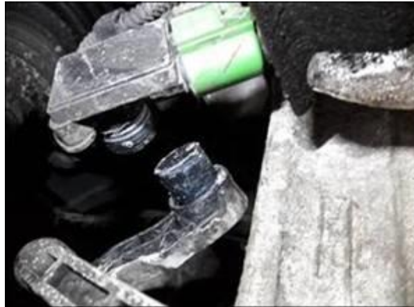
Figure 2. Possible damage of the self-leveling sensors.
