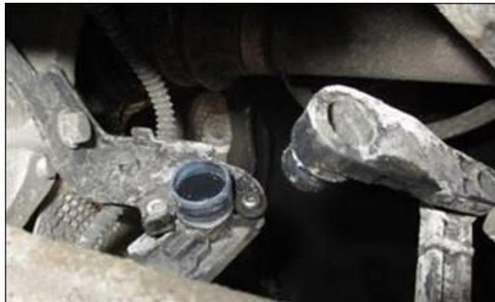
Figure 1. Possible damage of the self-leveling sensors.
