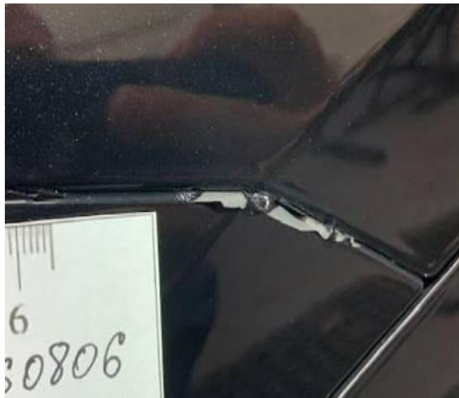
Figure 2. Paint peel on the bumper cover edge.
