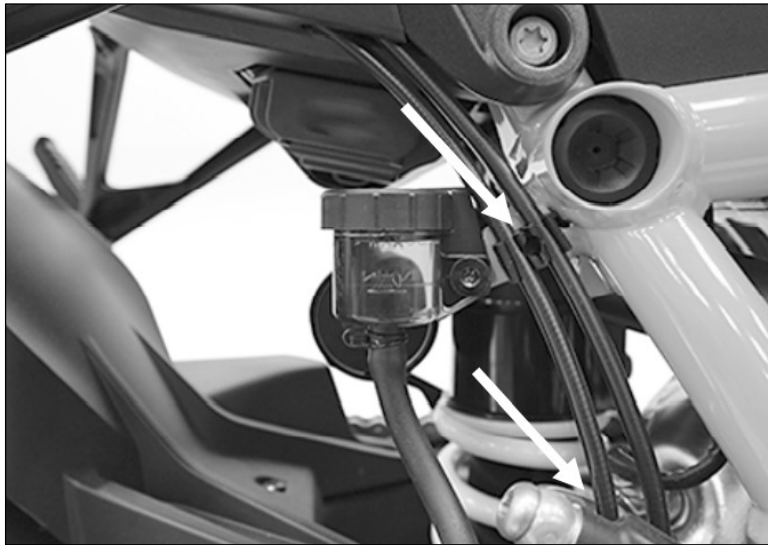
Fig. 1 – Cables in the area of the brake line
