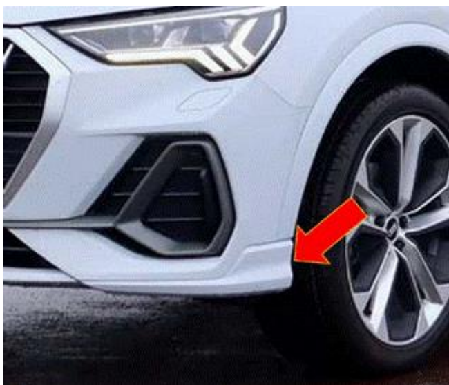
Figure 1. Location of paint peel on the front lower spoiler.
