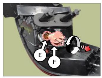
5. Remove the combination lamp wire harness from the tail lamp assembly. Use a pick to release the locking tab on the wire harness.
