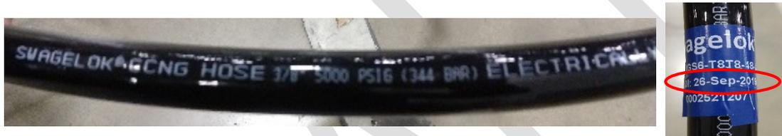
FIGURE 2-8. Left: Swagelok NG Series hose outer jacket marked “SWAGelok®” with size, rating for CNG fuel, pressure rating, and “ELECTRICALLY CONDUCTIVE”. Right: Swagelok hose decal includes date of manufacture (DOM) (circled).
