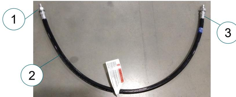
FIGURE 2-7. Swagelok NG Series hoses feature crimped collets (1), perforated polyurethane outer jacket (2), stainless steel ends (3).
