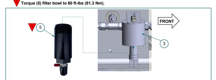
FIGURE 3-7. (5) retrofit HP fuel filter bowl, (3) HP fuel filter head
