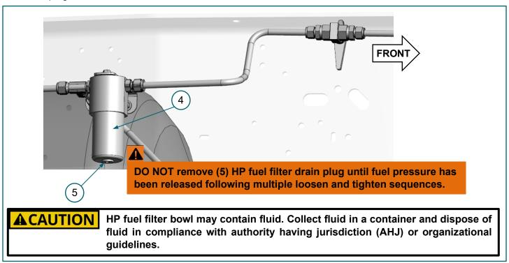
FIGURE 2-2. (4) HP fuel filter assembly, (5) drain plug
