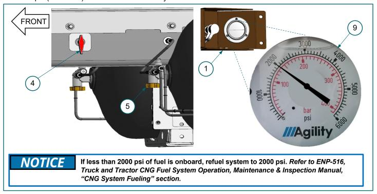
FIGURE 4-5. Fuel fill panel, (9) HP gauge reading 2000 psi, (4) 1/4-turn manual shutoff valve, (5) DS cylinder manual valve
