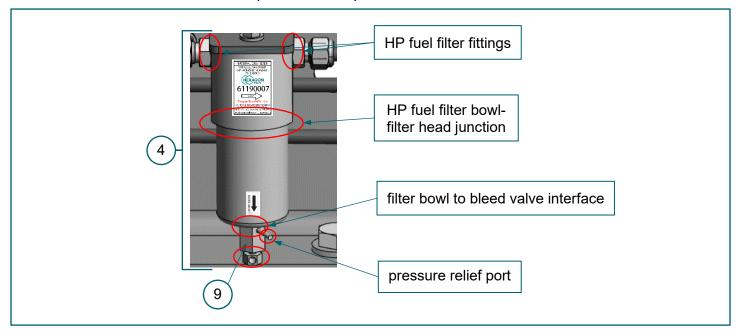
FIGURE 4-2. Apply leak detection fluid to (4) HP fuel filter assembly and (8) bleed valve at locations circled
