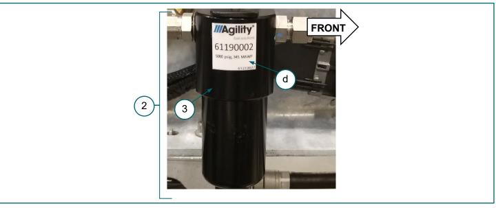
FIGURE 3-1. (2) high-pressure (HP) fuel filter assembly, (3) HP fuel filter head, (d) decal
