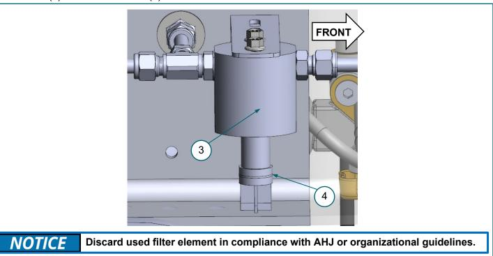
FIGURE 3-3. (3) HP fuel filter head, (4) filter element
