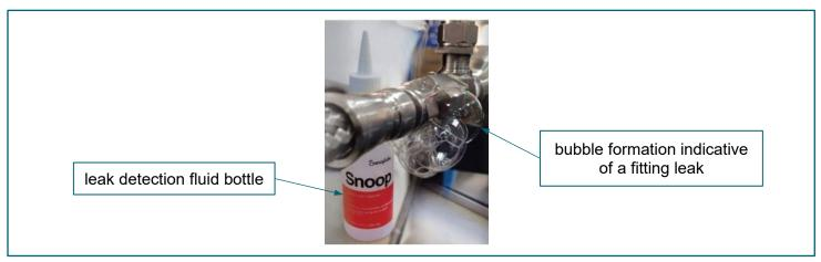
FIGURE 4-3. bubbles forming in leak detection fluid applied to a fitting junction
