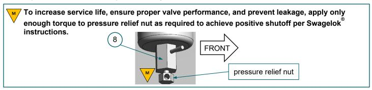
FIGURE 3-10. (8) bleed valve, pressure relief nut
