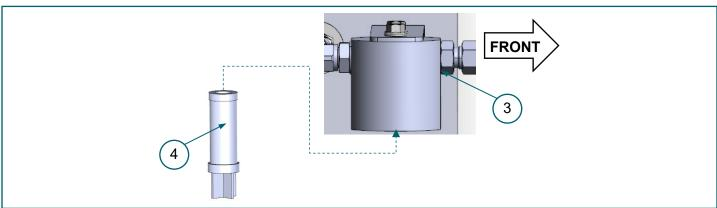
FIGURE 3-6. (3) HP fuel filter head, (4) filter element
