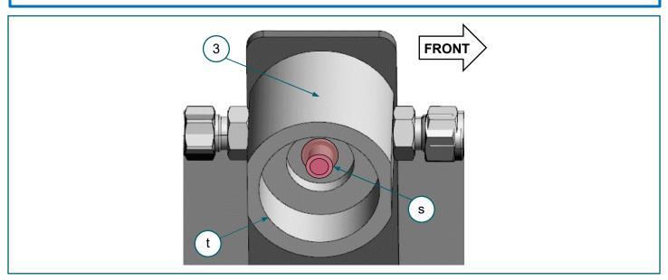
FIGURE 3-4. (3) HP fuel filter head, (s) filter element stem, (t) thread location
