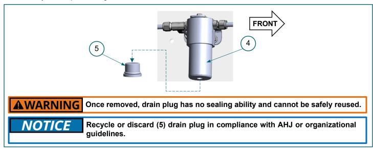
FIGURE 2-3. (4) HP fuel filter assembly, (5) drain plug (removed)
