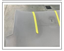
c. Inspect the condition of the headliner after the 1<sup>st</sup> round of cleaning. The headliner should have no visible staining remaining.
