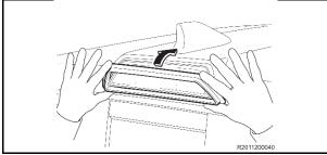
b. Hold the trim ring as shown in the illustration and apply it straight onto the vehicle making sure to center it on the center high mount stop lamp.
