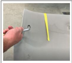
b. Using a Compressed Air Nozzle, blow air across the effected area at a 30 degree angle to prevent damage. Blow across the headliner until it's dry, which should take approximately 30 seconds for a 12"x12" area.
