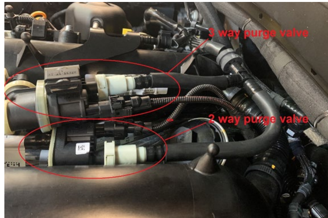
Figure 1: - High load purge line on V8 engine.
