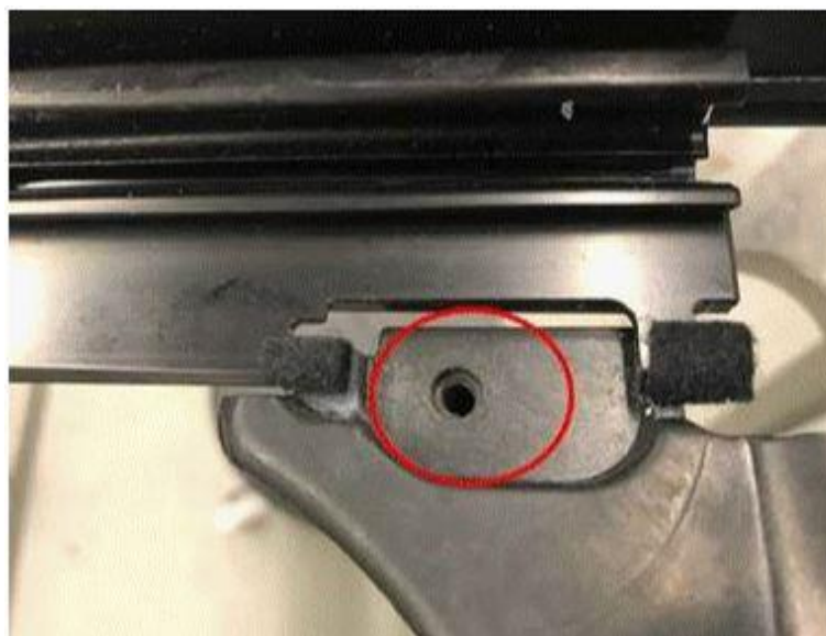
Figure 10. Apply thread locker in this area.
