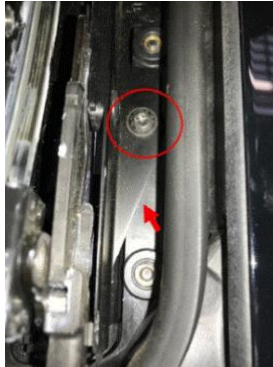
Figure 16. Location of rear guide rail bolt and area to be lifted with a plastic wedge.
