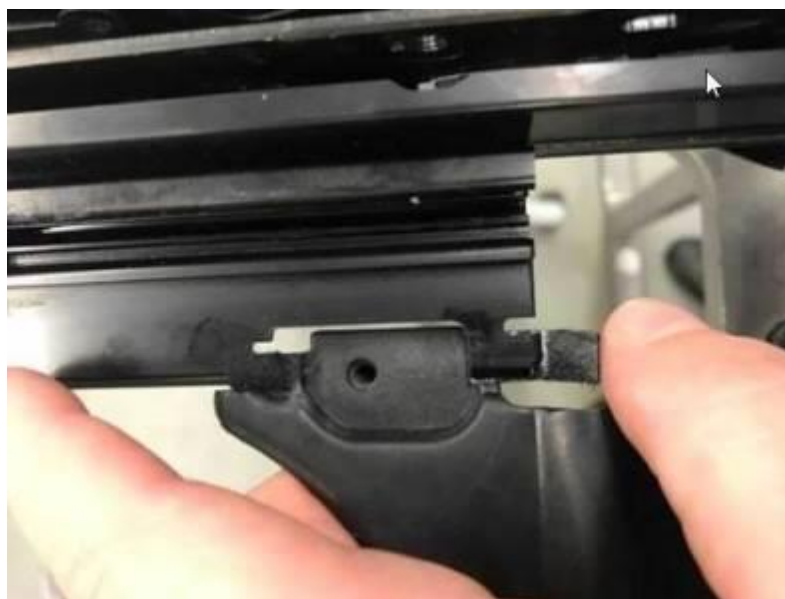
Figure 8. Applying felt tape.
