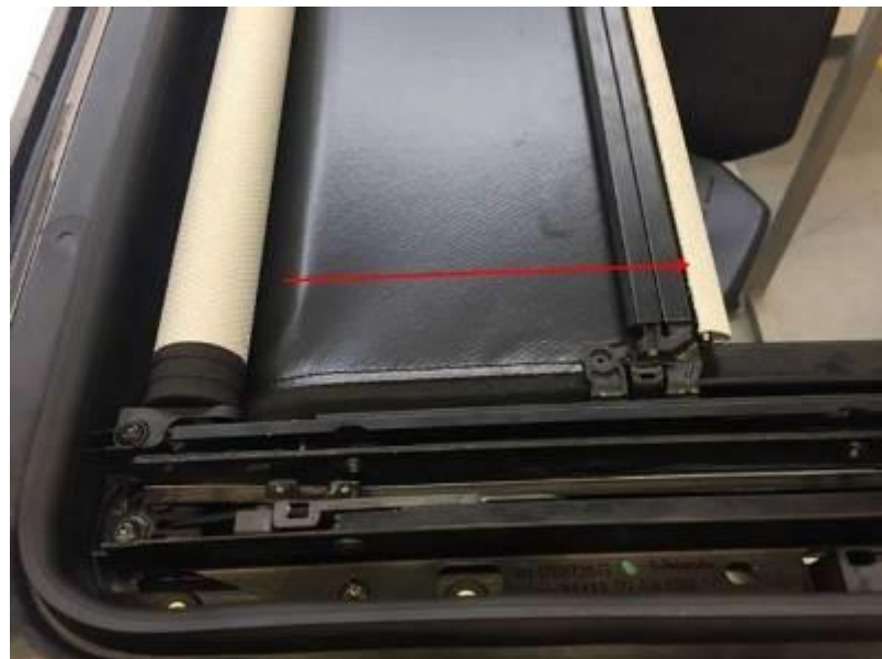
Figure 1. Closing the roller shade.
