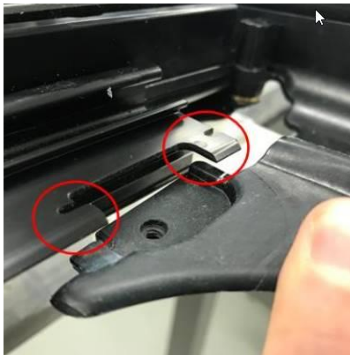
Figure 7. Areas to clean using cleaning solution D 009 401 04.
