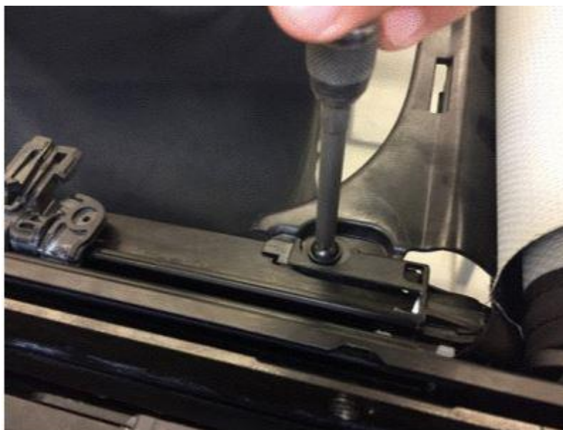
Figure 11. Torque screws to 3Nm.
