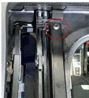
Figure 12. Loosen the bolt a few turns but do not remove the screw completely.
