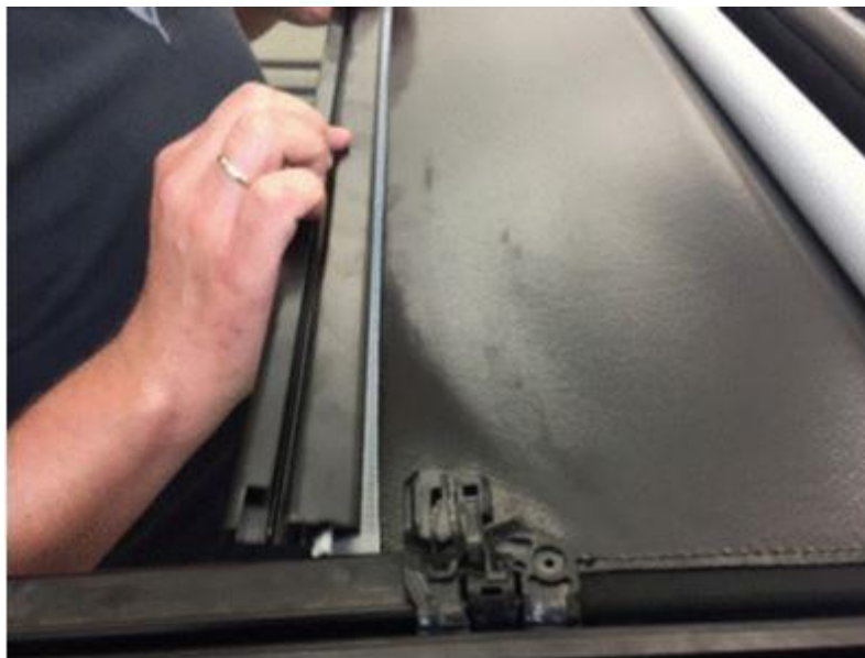
Figure 3. Beam removed from the drive.
