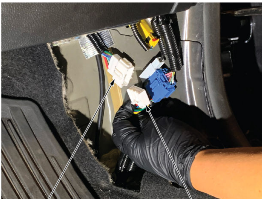
ENGINE ROOM HARNESS CONNECTOR Disconnect.
