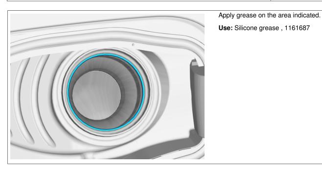
Apply grease on the area indicated. **Use:** Silicone grease , 1161687
