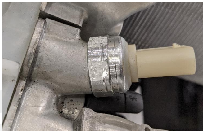
Figure 13 – P/T sensor properly seated
