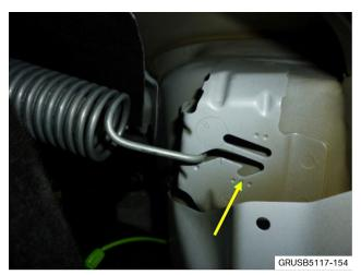
5. Ensure the spring is attached to the rearmost hook (shown by the arrow). If it is, continue troubleshooting, this bulletin does not apply.
