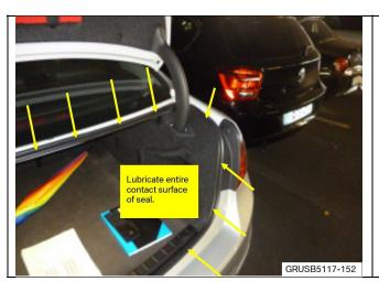
2. Once dry, apply Carbaflo lubricant P/N 83 23 0 309 627 to the entire seal.
