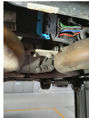
Figure 8: Position of the X090 connector for the current measurement absorbed by the compressor during the actuations.
