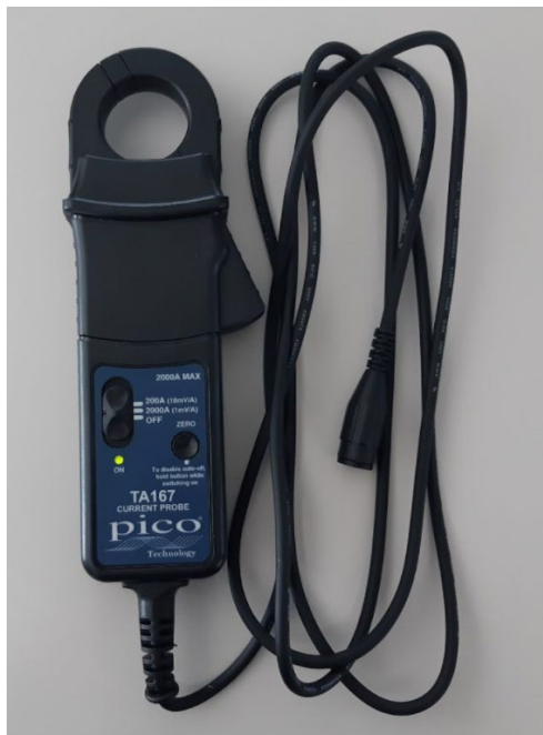
Figure 11: Current clamps to be used for the measurement of current absorbed by the compressor.
