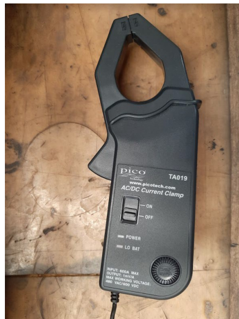
Figure 11: Current clamps to be used for the measurement of current absorbed by the compressor.
