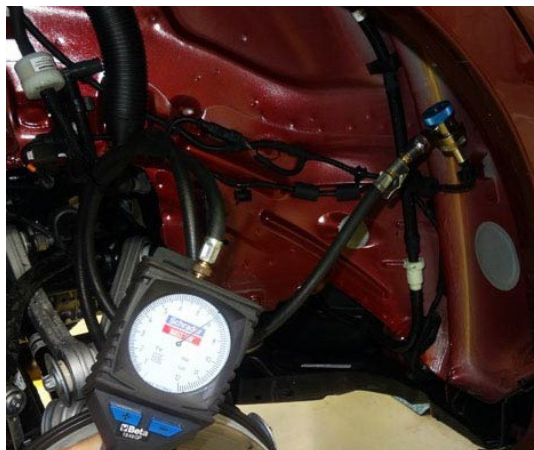
Figure 1: Measuring the pressure of the air suspension system using a pressure gauge.
