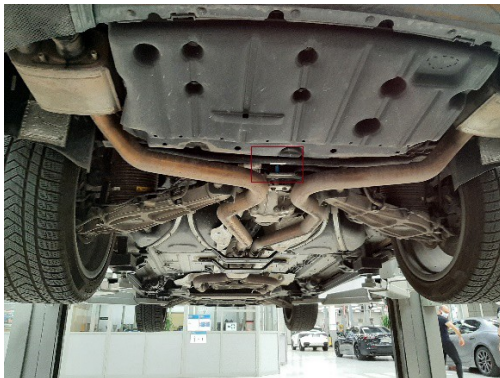
Figure 8: Position of the X090 connector for the current measurement absorbed by the compressor during the actuations.
