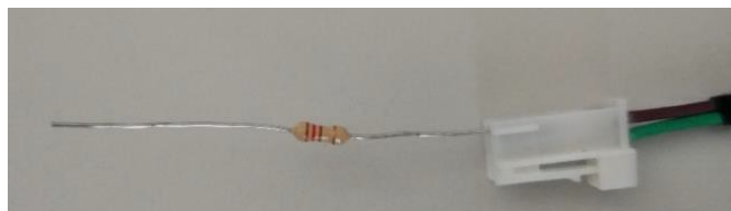
Figure 4: Example of connector and resistor for the drag test.
