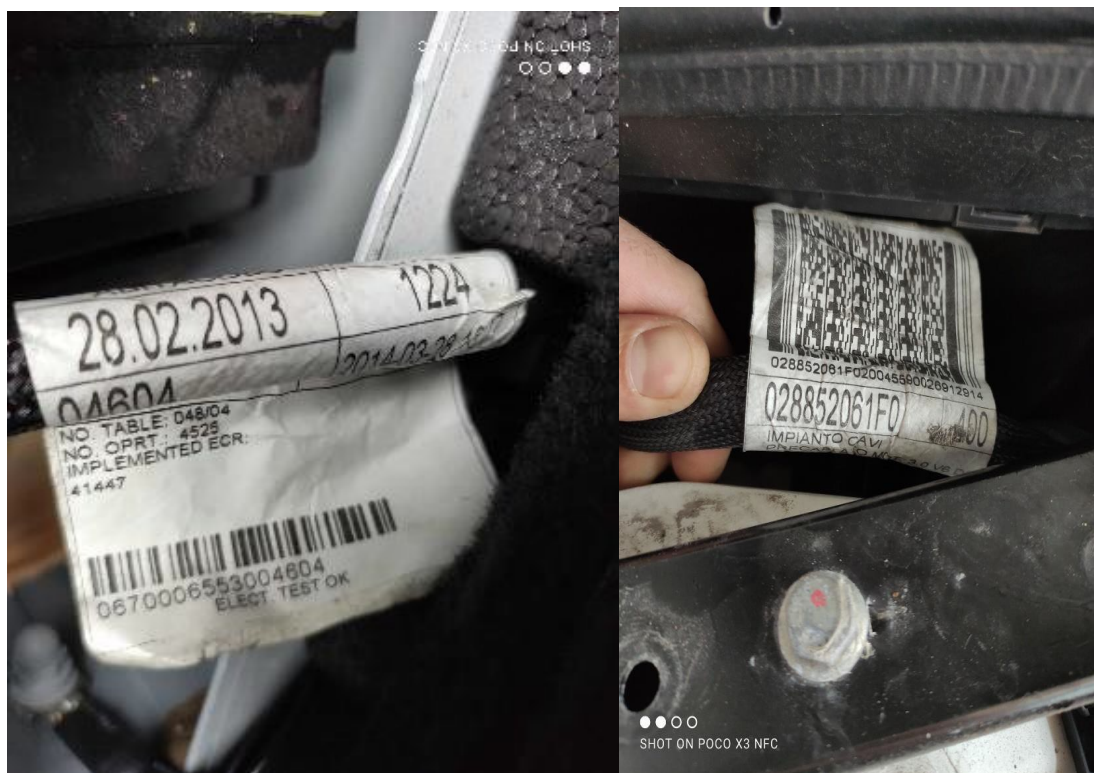
Figure 2: Examples of the Traceability Labels of the Battery Positive Wiring (left) and the Recharge Wiring (right).
