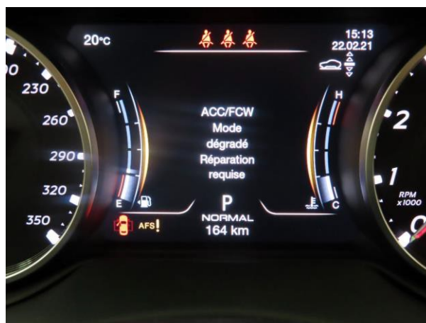
Figure 1: Possible warning message related to one of the ADAS systems linked to the HALF module.
