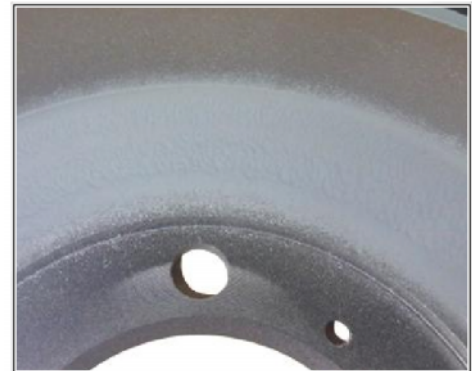
Brake disc with corrosion protection
