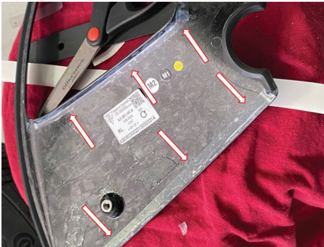
Figure 2 - Edges for Teflon/Felt Tape Application
