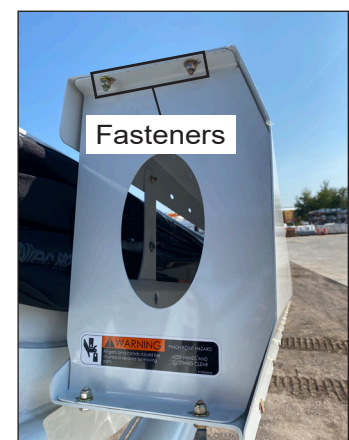
Figure 4 – Removing Rear Fasteners
