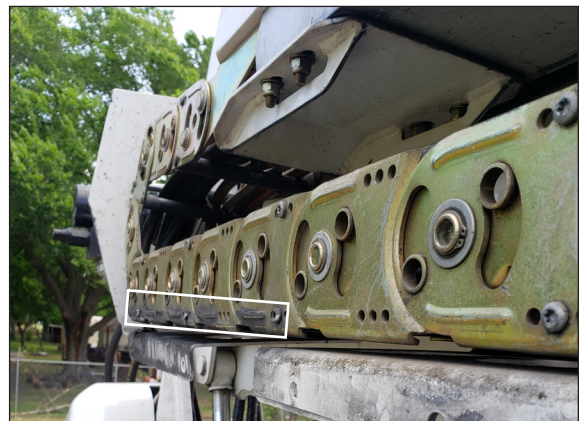
Figure 10 – Scraped Links, Damaged Screws
