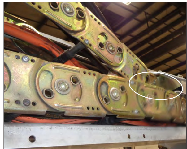
Figure 14 – Bent Links and Mounting Foot
