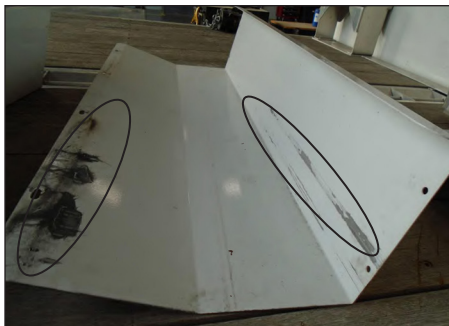
Figure 8 – Cover Damage Examples
