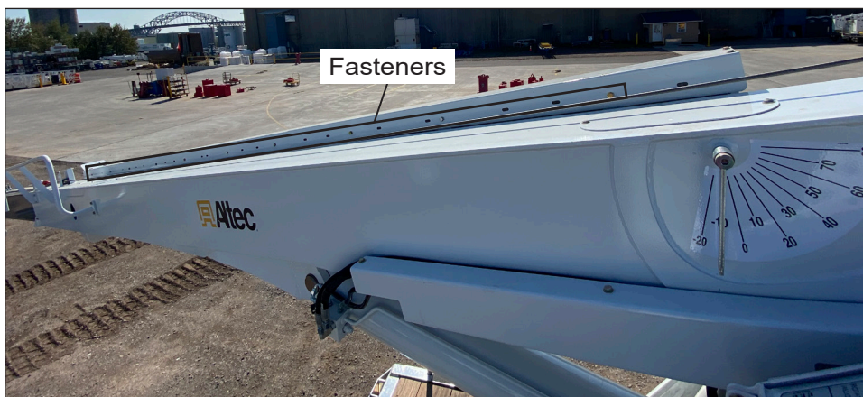
Figure 3 – Removing Top Fasteners
