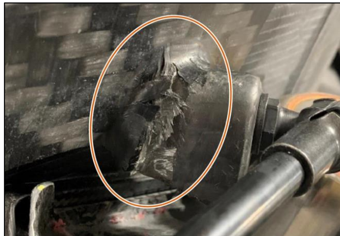
Example of substrate failure
