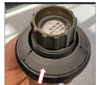
Figure 6 Application of Grease to Centerlock Cone
