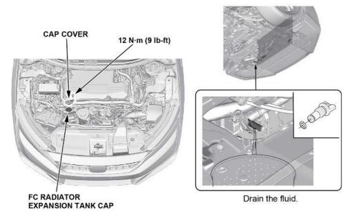
8. Remove the DT radiator expansion tank cap and drain the DT coolant.
