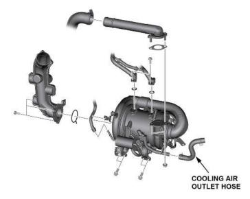
37. Remove the rear mount mounting bolts from the FC stack.
