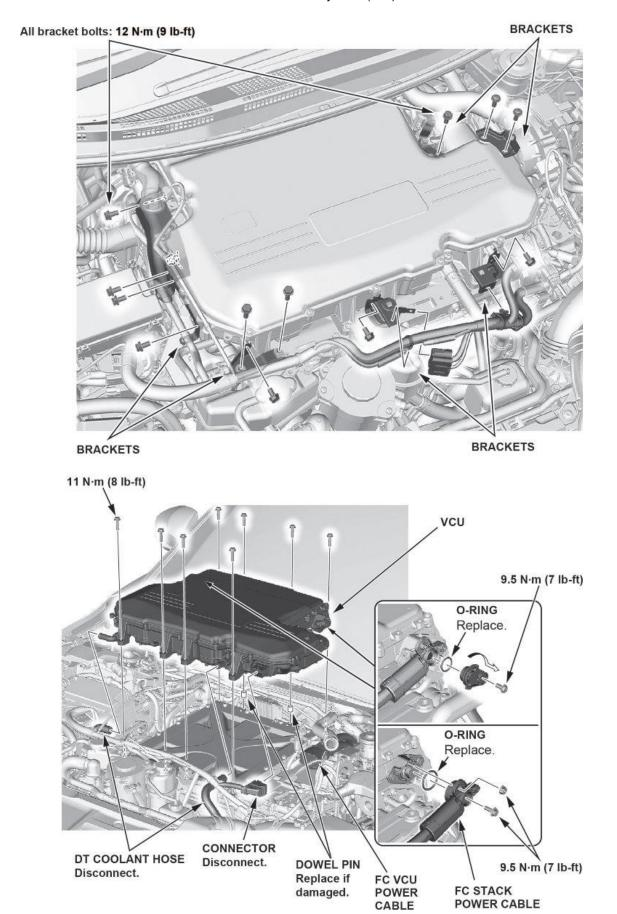
NOTE: The marks located on the back of the FC VCU show which bolts to remove.
