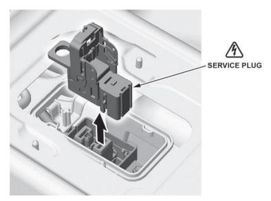
17. Wrap the service plug base with insulating tape.
