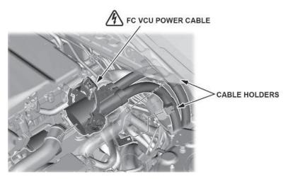
19. Remove the left and right FC stack power cable cover.
