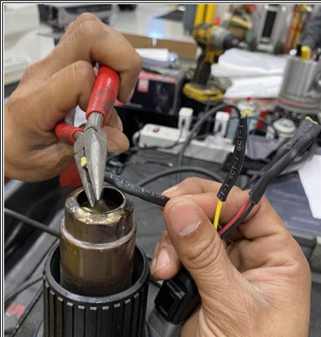
6. Use a heat gun to apply heat to each piece of heat shrink tubing, ensuring glue is extruded from the end and sealed by pinching the end of each piece with pliers (Refer to figure #7).
