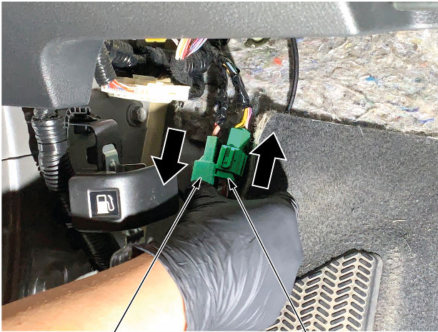
ENGINE ROOM HARNESS CONNECTOR Slide apart.
