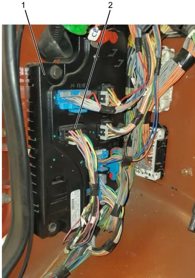
Figure 2. Body Control Module (BCM) Harness and Connectors
