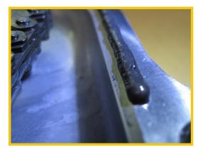
**NOTE:** As shown above, a properly applied, small bead of sealant will fill in the chamfered portion after the cover is installed. Do not use an excessive amount of sealant.
