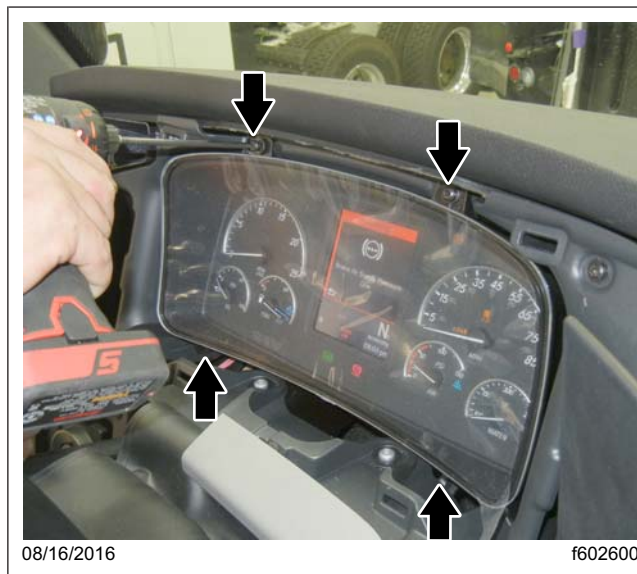
Fig. 5, ICUC Mounting Screws
