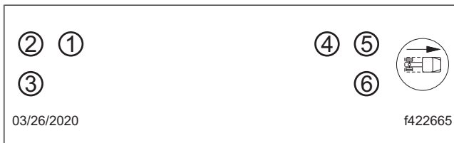
Fig. 4, Tightening Pattern, Left-Front Axial Caliper
