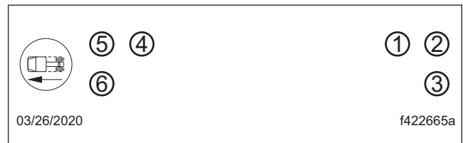
Fig. 5, Tightening Pattern, Right-Front Axial Caliper
