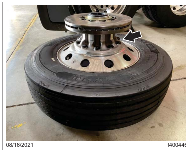
Fig. 1, Hub Held in Place on Front Wheel
