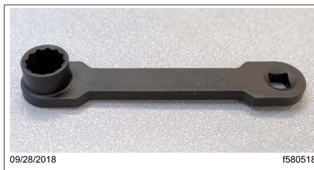
Fig. 3, DDC DSNCHA018005 30 mm Air Disc Brake Caliper Brake Bolt Torque Adaptor
