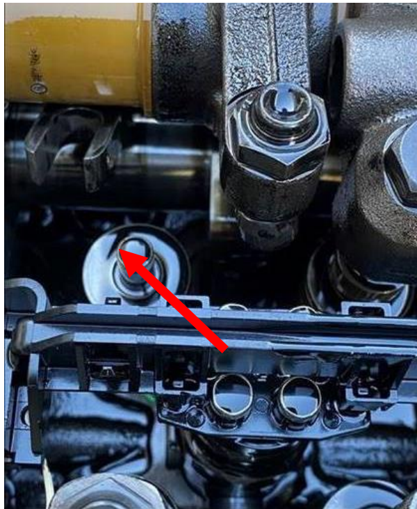
Figure 1. Exhaust Valve Bridge Out of Position
