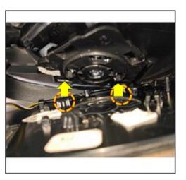
b. Press the hooks (orange circles) on the upper side of the mirror holder into the holes of the pivot plate.
