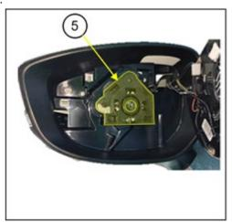
5. Peel off the release papers (1) on the mirror glass holder (2).
