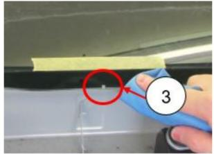
5. Align the middle of the protection film to the marking on the windshield and place it within 2 mm of the bottom of the windshield.
