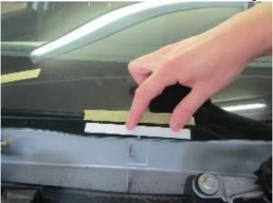
6. Align the mark (3) and middle of protection film (4) on the dotted red line.
