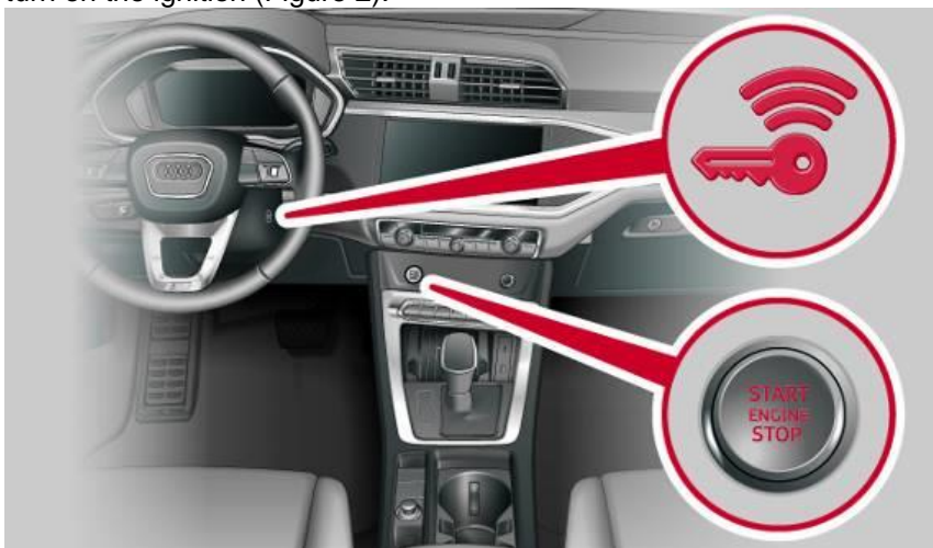
Figure 2. Key reader coil location.
