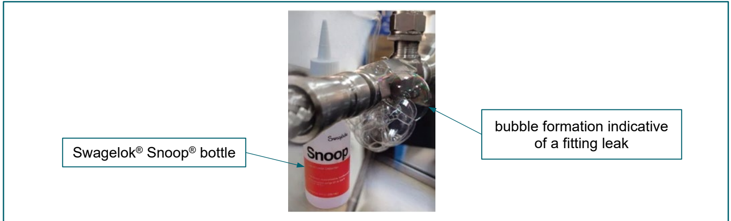
FIGURE 4-3. Swagelok® Snoop®, bubbles forming at a fitting junction
