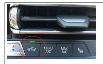
1. Activate the air recirculation function by pressing the recirculation button on the climate control panel (Recirculation mode, circled), LED ON. This will close the top fresh air flap leaving the bottom two recirculation flaps open.
