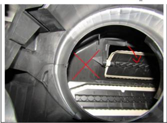
6. If the flap system is not OK, try to correct the flap by hand. See direction of arrow.
