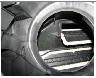
5. Check correct position of the fresh air flap through the blower motor opening, or using a borescope from the microfilter opening (NOTE: This flap is the top of three flaps).
