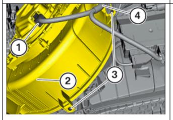
4. Remove the ventilation system blower motor.
