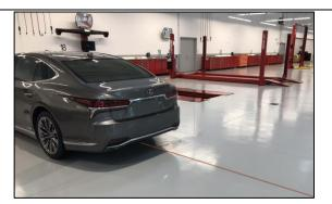
B. Creating a Centerline Using a 90-Degree Laser (for Forward Recognition Camera and Front Millimeter Wave Radar)
