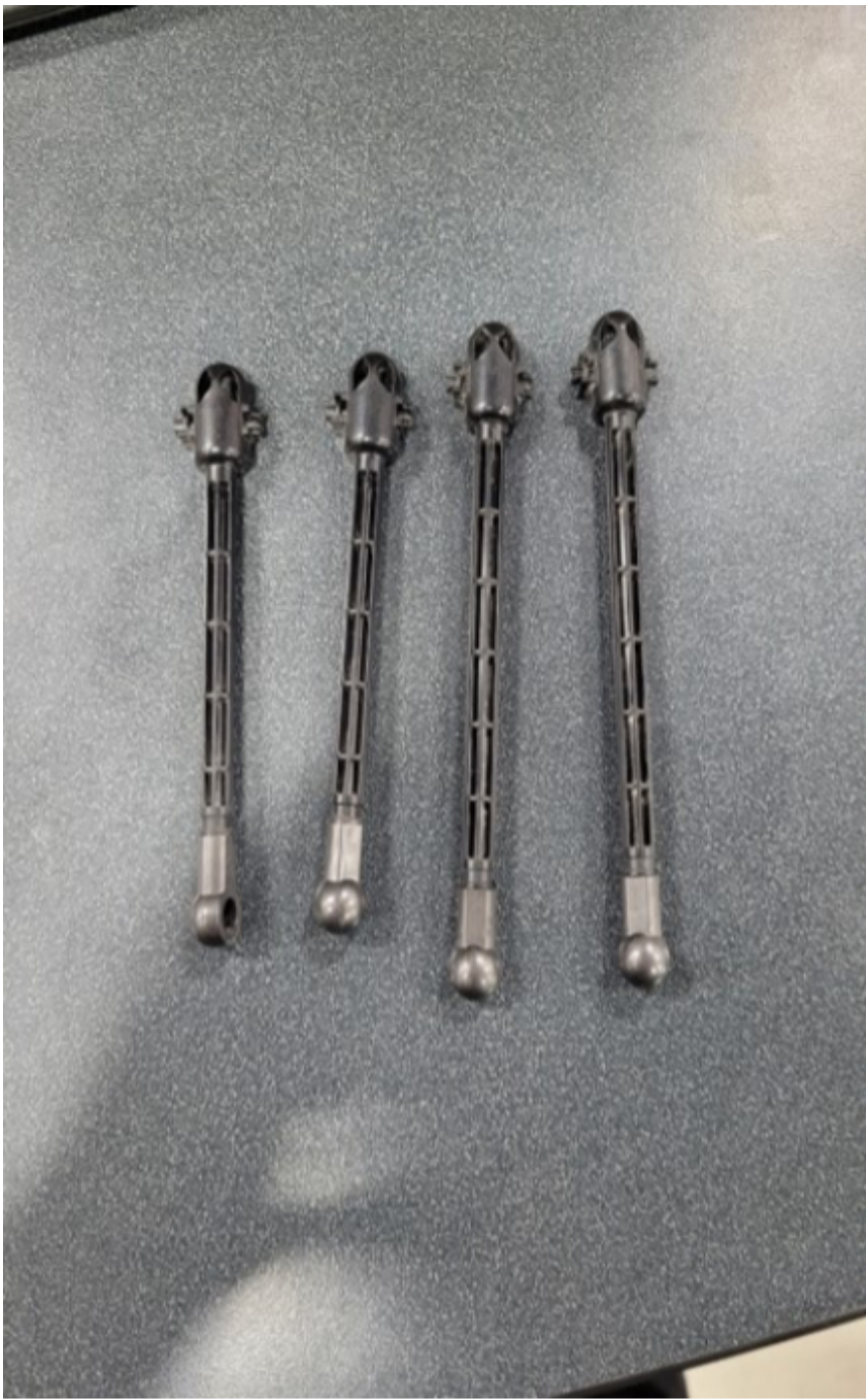
Aftermarket Adjustable suspension height sensor links. As shown below:
