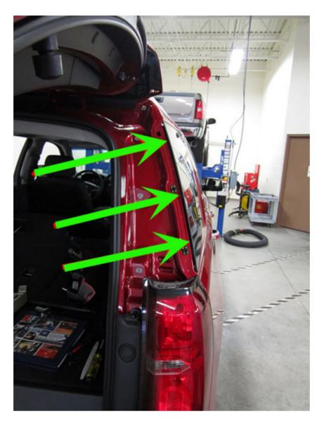
2. The gap between the rear tail light assembly and the quarter panel, as shown below.
