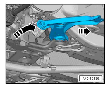
• Check left front and right front lower control arms and replace if necessary.
