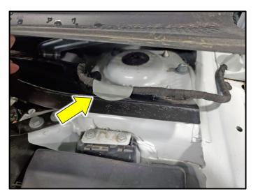
Reinstall cable holder onto longitudinal member as shown.
