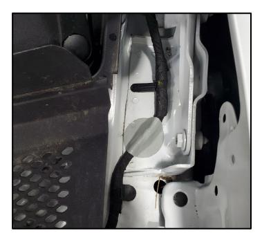
Reroute wiring harness for the heated washer jets.
