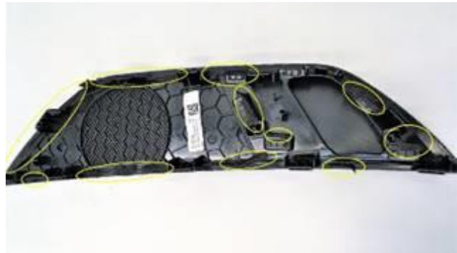
Figure 2. All tabs on the midrange speaker trim that require felt strip material.
