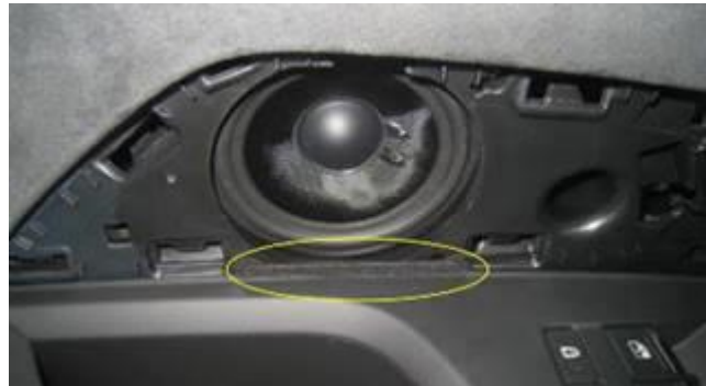
Figure 1. Felt strip section applied to opening in door panel.
