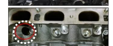
4. Upon removal of the GDI Injector, if injector has the appearance as seen to the right, replace the whole injector. Do not just replace the tip seal of the injector in this case.
