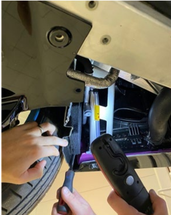
HVAC pipes and unions behind left hand wheel arch liner
