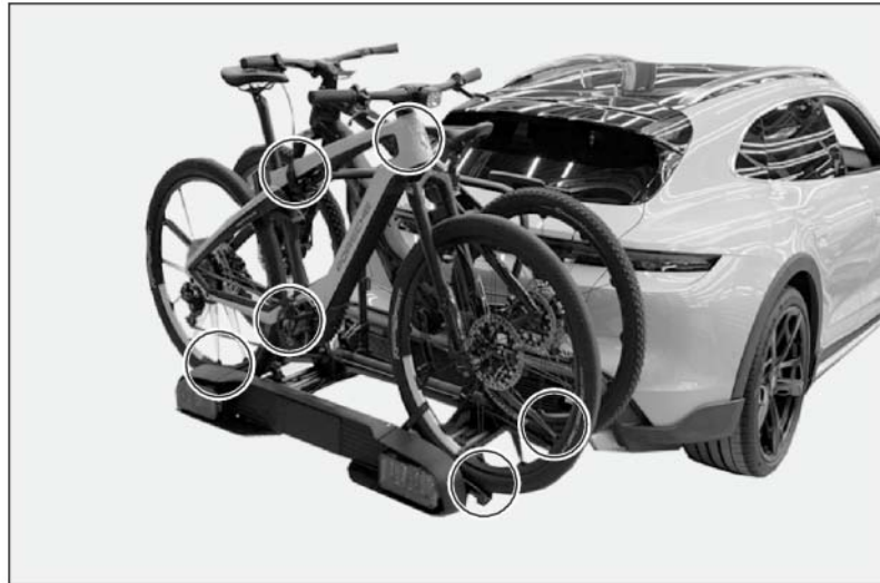
Overview of ratchets for tensioning points on the bike
