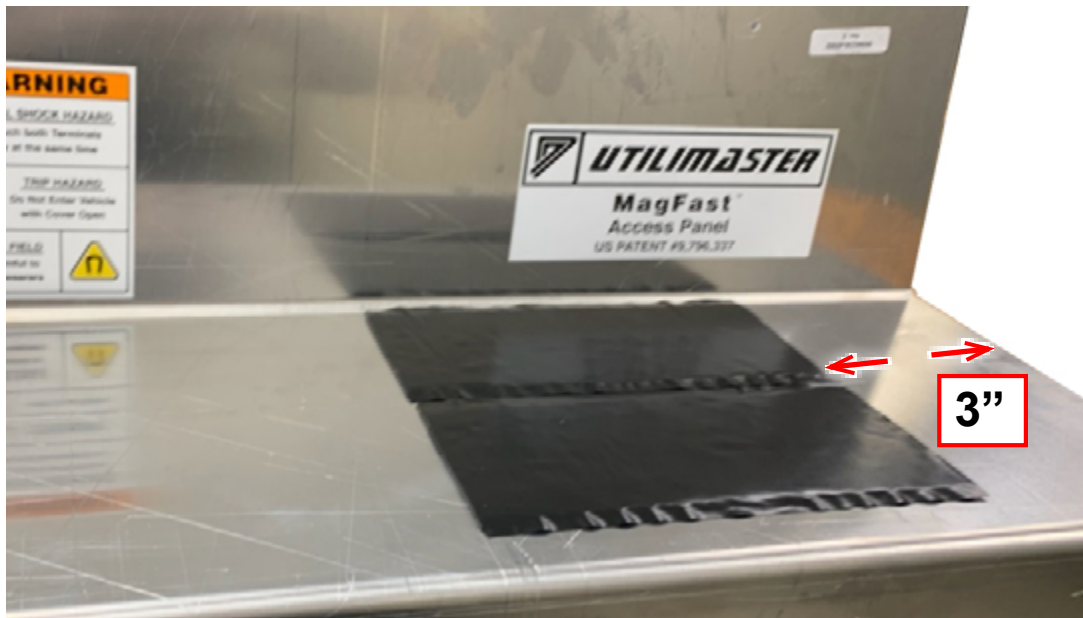
Vinyl tape applied to underside of the stepwell lid
