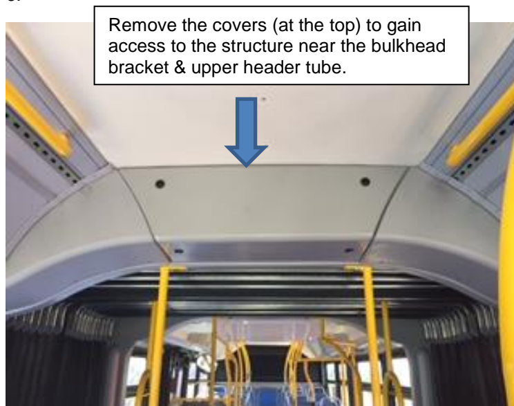
FIGURE 6: SHOWN INTERIOR COVERS TO BE REMOVED TO GAIN ACCESS
