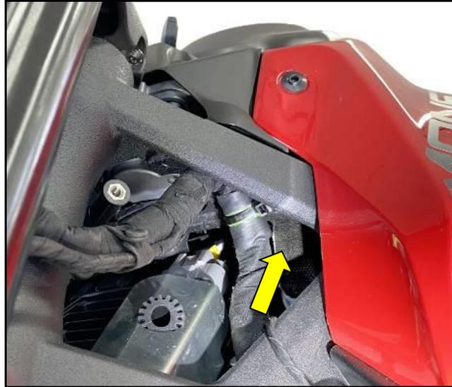
7. Tighten tie to fasten wiring in its position
