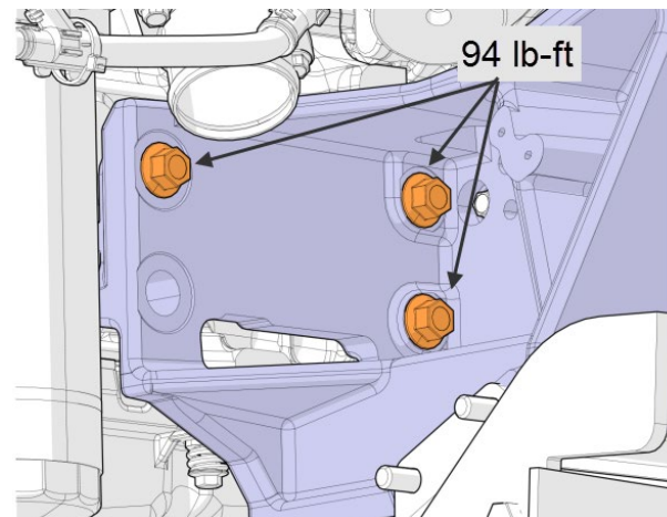
FIGURE 58: THREE (3) SCREWS ON THE SIDE OF THE ENGINE MOUNT
